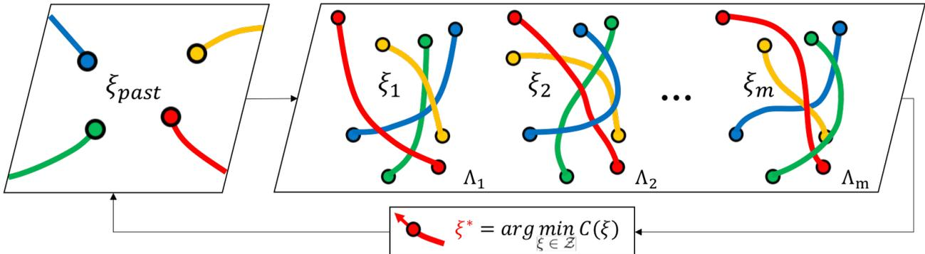
Fig. 1: Pictorial representation of the Topologically Adaptive Navigation Planning scheme. The robot observes agents’ past trajectories  $\zeta$ , generates a set of  $m$  possible scene evolutions  $\Lambda_1, \dots, \Lambda_m$ , derives geometric representations of them  $\xi_1, \dots, \xi_m$  and picks the next action assigned to it from the trajectory of the lowest cost,  $\xi^*$ .
