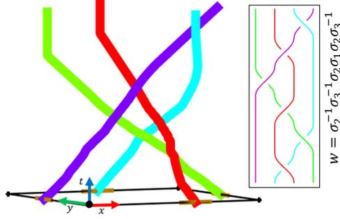
Fig. 3: Projecting a trajectory collection (left) to the  $x$  axis to derive a braid diagram and a braid word (right). The visualization of the braid diagram and the extraction of the braid word was done using BraidLab [22].
